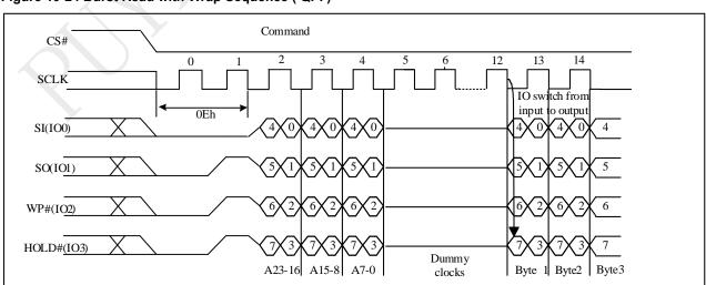
Figure 10-24 Burst Read with Wrap Sequence (QPI)
