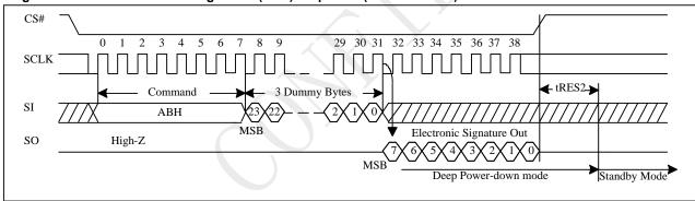
Figure 10-43a Read Electronic Signature (RES) Sequence (QPI)
