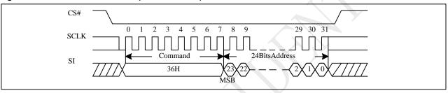
Figure 10-52a Individual Block Lock(QPI)
