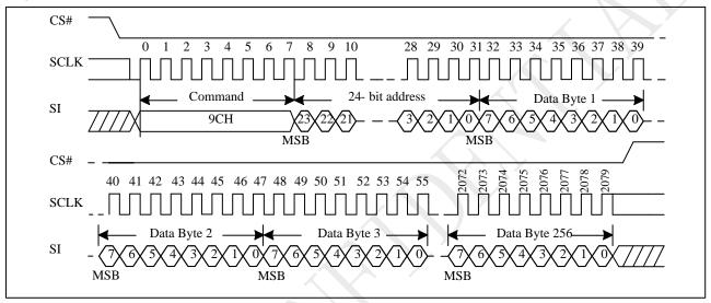
Figure 10-37a Buffer Write Sequence (QPI)
