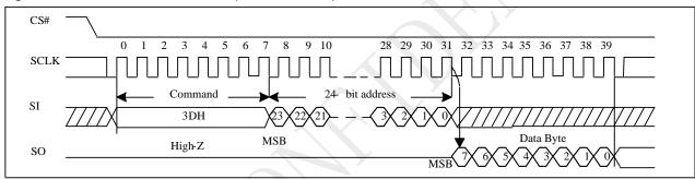
Figure 10-54a Read Block Lock Status (QPI)
