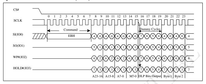
Figure 10-25c DTR 4IO Read with DLP bits output Sequence
