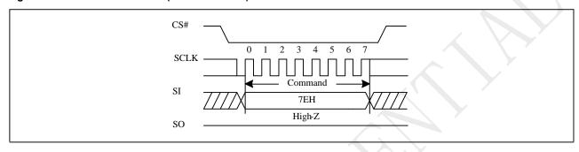
Figure 10-55a Global Block Lock(QPI)
