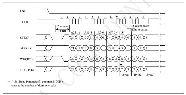
Figure 10-18a 4IO Read in QPI mode Sequence (QPI M5-4 ≠ (1,0))
