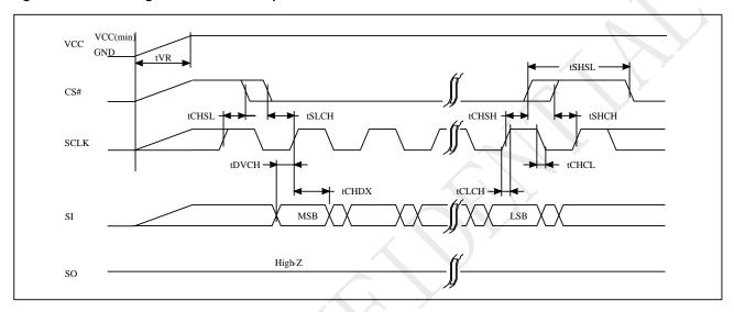
Figure 5-9 Power-up Timing
