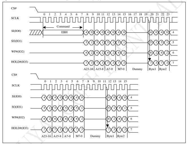
Figure 10-18b 4IO Continuous Read Sequence (M5-4 = (1,0))
