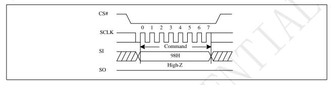
Figure 10-56a Global Block Unlock(QPI)
