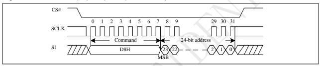
Figure 10-31a Block Erase (BE) Sequence (QPI)
