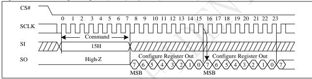
Figure 10-6a Read Configure Register (RDCR) Sequence (QPI)
