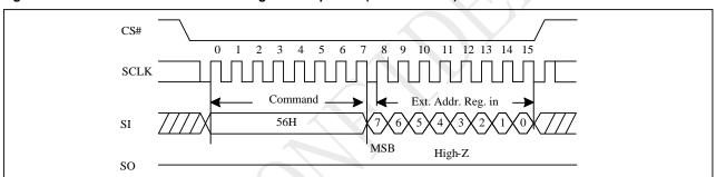
Figure 10-10 Write Extended Address Register Sequence (Command 56)
