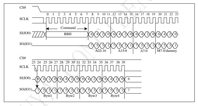
Figure 10-15 2IO Read Sequence (Command BB M5-4 ≠ (1,0))
