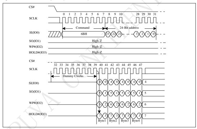
Figure 10-17 Quad Read Sequence (Command 6B)
