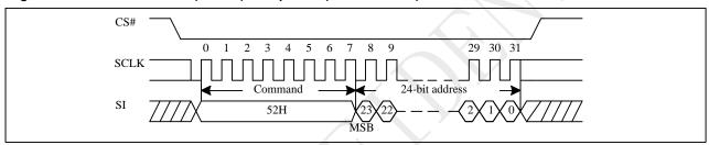
Figure 10-30a Block Erase 32K(BE32K) Sequence (QPI)
