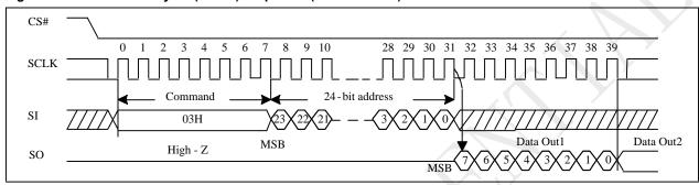
Figure 10-11 Read Data Bytes (READ) Sequence (Command 03)
