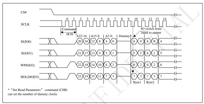
Figure 10-23 Burst Read with Wrap Sequence (QPI)
