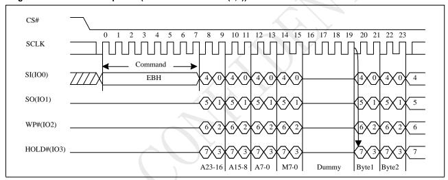
Figure 10-18 4IO Read Sequence (Command EB M5-4 ≠ (1,0))
