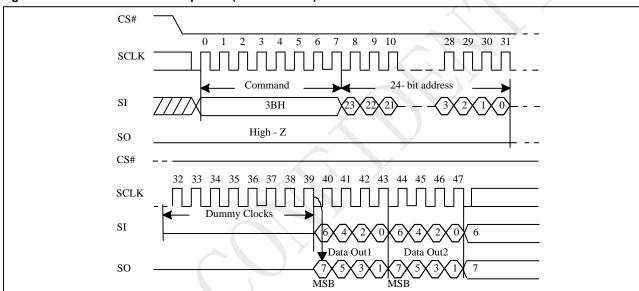
Figure 10-14 Dual Read Mode Sequence (Command 3B)
