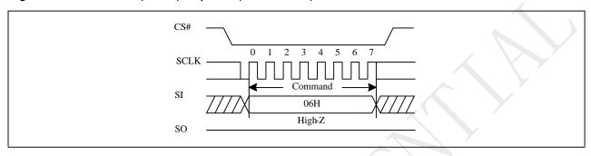
Figure 10-2a Write Enable (WREN) Sequence (QPI)
