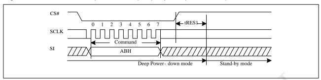
Figure 10-43c Release from Deep Power-down (RDP) Sequence (QPI)
