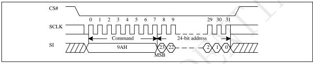
Figure 10-35a Buffer Load Sequence (QPI)
