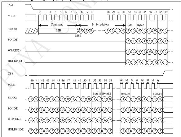
Figure 10-34 Quad Page Program (QPP) Sequence (Command 32)
