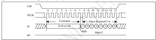
Figure 10-7a Write Status Register (WRSR) Sequence (QPI)
