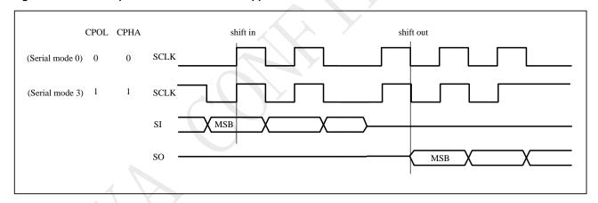
Figure 8-1 Serial Peripheral Interface Modes Supported
