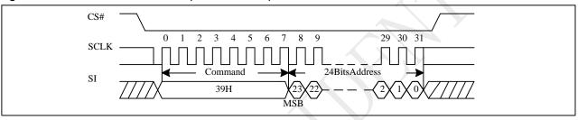
Figure 10-53a Individual Block Unlock(QPI)
