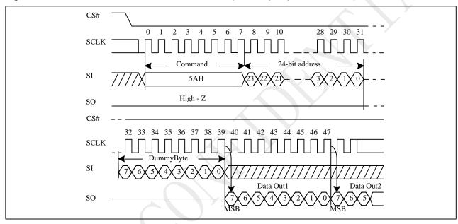
Figure 10-60a Read Serial Flash Discoverable Parameter (RDSFDP) Sequence(QPI)
